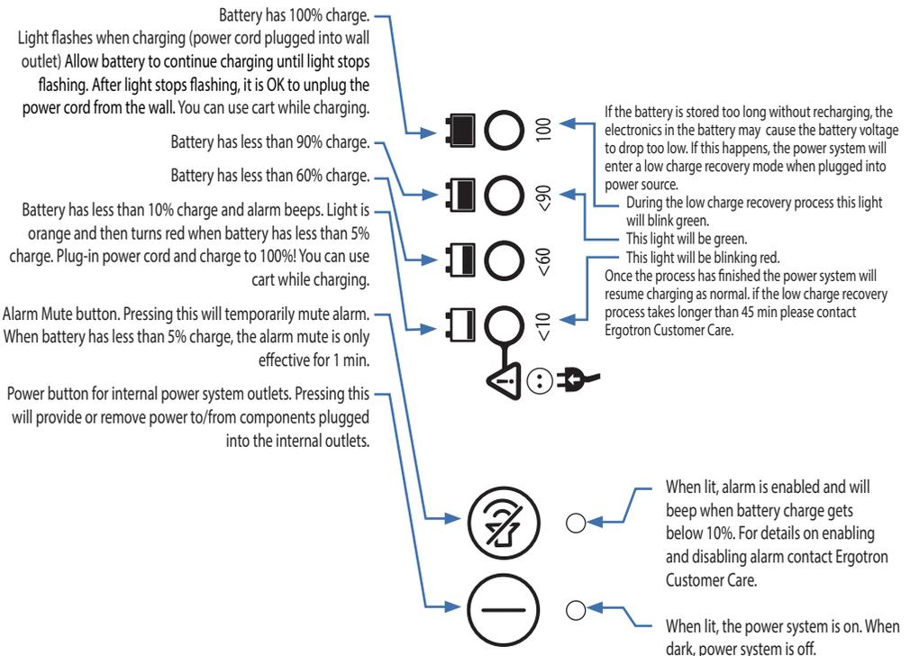
**If other lights are flashing red/green it could indicate a power system fault. If this occurs contact Ergotron Customer Care.**
